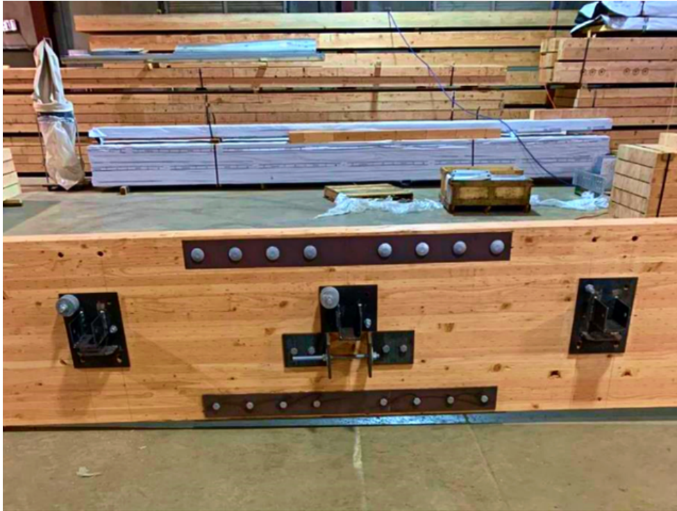
Connections are pre-assembled in our plant in Jefferson, Oregon.
