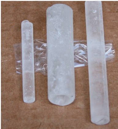
Sample of Diffuser Rods showing different sizes.
